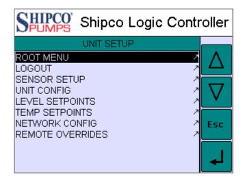
**WARNING:** Be cautious adjusting parameters in Unit Setup! Certain parameters are factory set to design specifications and incorrectly adjusting these parameters could result in unit malfunction and/or serious equipment damage. Consulting the factory or local service representative is highly advised before making adjustments which could affect unit operation.
