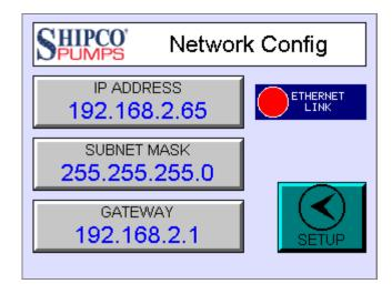
BACnet IP requires physical connection to the 10/100 Mbps Ethernet (LAN) port on the controller and communication occurs via UDP port 47808 (0xBAC0).
