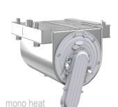
DynaMax models 210-250 feature a MONO design heat exchanger wherein the secondary heat exchanger is separated by a divider plate from the primary heat exchanger.
