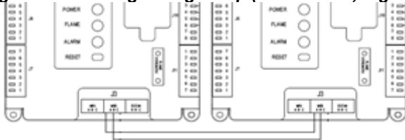
Figure 33: Lead lag Wiring Setup (Left: Master, Right: Slave)
