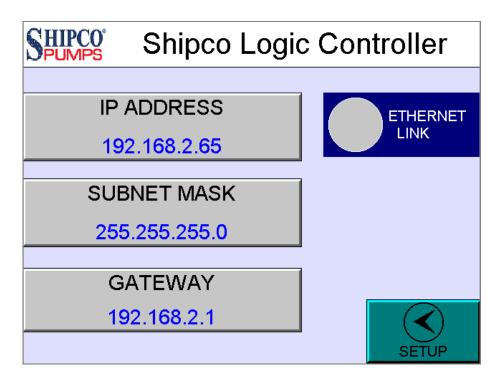
BACnet IP requires physical connection to the 10/100 Mbps Ethernet (LAN) port on the controller and communication occurs via UDP port 47808 (0xBAC0).
