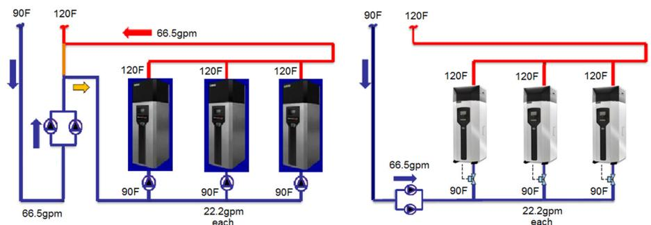
Comparison 3: Primary-Secondary vs. Primary-Only on 30°F (16.7°C) System ΔT
