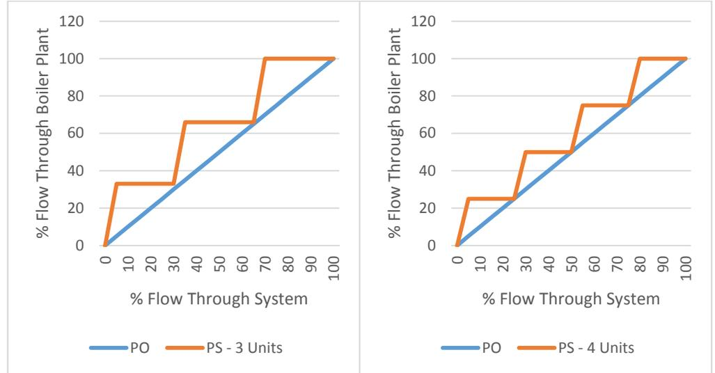
Constant Speed Boiler Pumps vs. Variable Speed System Pump
