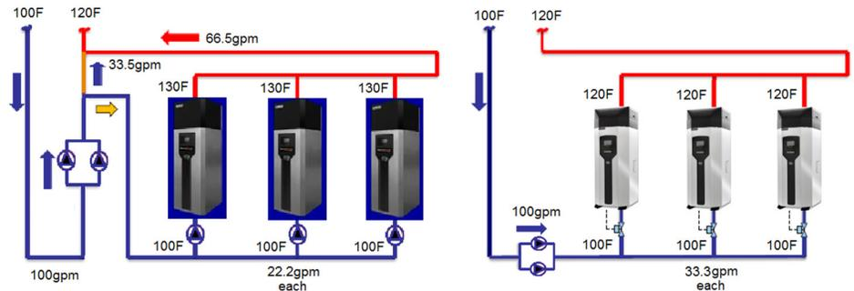
Comparison 2: Primary-Secondary vs. Primary-Only on 20°F (11.1°C) System ΔT
