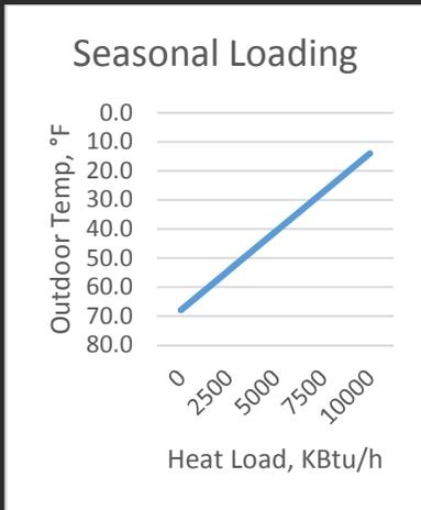
The reason for this is that cooler weather means a greater differential between the fluctuating temperature outdoors, and the target room temperature, which is static. As the difference between these two grows, heat is lost through the building envelope with increasing speed, meaning that more Btu's need to be added every hour.
