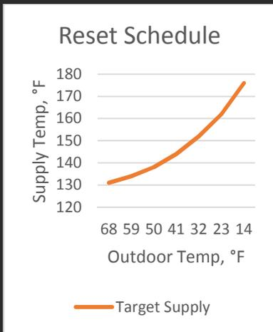
In principle, systems with outdoor reset use the same flow rate for all loads, but they cool the water more during higher demand, meaning the  $\Delta T$  varies according to the load.
