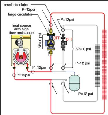
Step 2: The 10psi pump activates. High pressure drop ( $\Delta P$ ) on the boiler heat exchanger creates a 5psi  $\Delta P$  across the supply/return header. The small pump will not be able to overcome it, meaning no flow.
