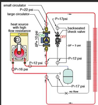
Step 3: Hydraulic separation reduces common piping  $\Delta P$  so both system loops function. A pump is added to create flow through the boiler.
