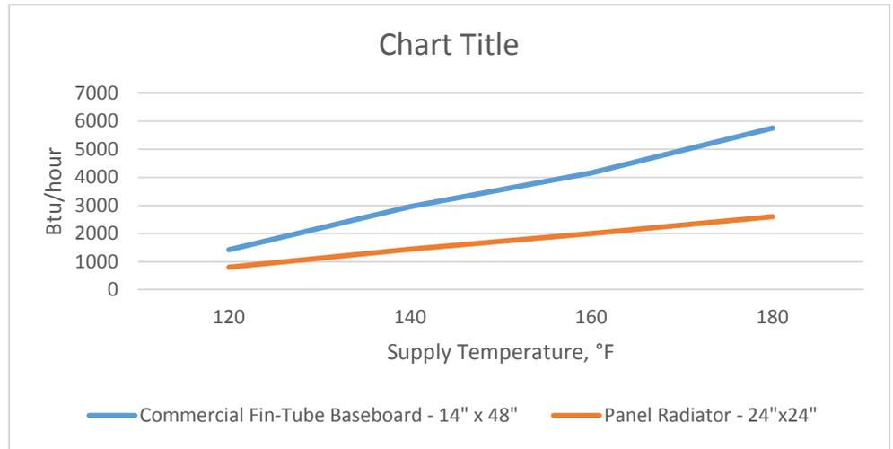
For example, 1gpm fed through 10' of fin-tube baseboard at 160°F (71.1°C) will deliver 10.4 KBtu/h and be 20.8°F (11.5°C) colder when it exits the baseboard. The same 1gpm fed at 140°F (60.0°C) will deliver 7.4 KBtu/h and be 14.8°F (8.2°C) cooler.
