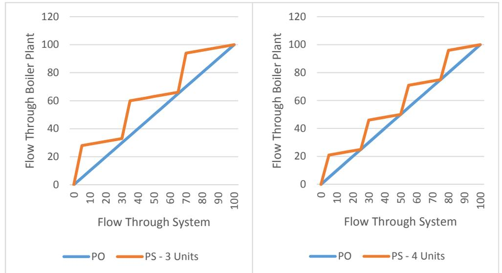
Variable Speed Boiler Pumps vs. Variable Speed System Pump
